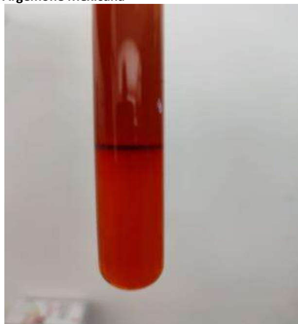
Figure 1: Ring formation in Nitric Acid Test for Argemone Mexicana
